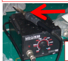
Oxidation. Poor maintenance.
